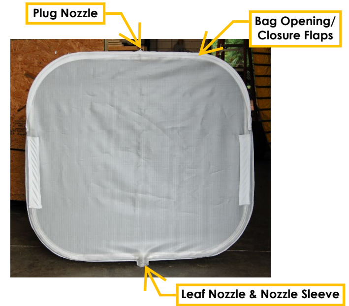
Figure A | Leaf bag installed on filter leaf. Note that the closure flaps and plug nozzle are located on the top of the leaf when oriented vertically.
