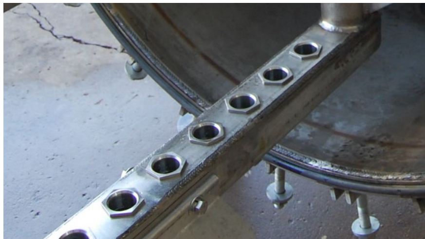
Figure B | Inserts after being installed in manifold
